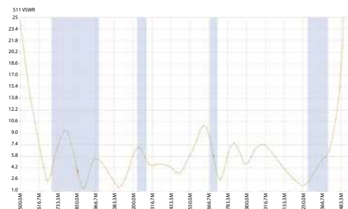
AN-E antenna measurement graph
