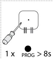
Bypressing the programming button on the actuator for 8 seconds, deletion of one transmitter activates. LED flashes 4x in each 1s interval. Pressing the required button on the transmitter deletes it from the actuator's memory. To confirm deletion, the LED will confirm with a flash long and the component returns to the operating mode. The memory status is not indicated. Deletion does not affect the pre-set memory function.
