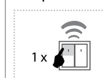
The output contact will be closed by pressing the button and opened by releasing the button. For the correct execution of individual commands (press = closing / releasing the button = opening), the time delay between these commands must be a min of. 1s (press - delay 1s - release).
