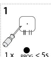
Press of Prog button for 3-5s will activate actuator RFSA-62B into programming mode. LED is flashing in 1s interval.
