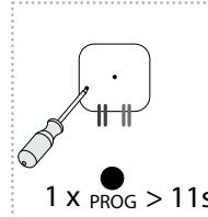
By pressing the programming button on the actuator for 11 seconds, deletion occurs of the actuator's entire memory. The actuator goes into the programming mode, the LED flashes in 0.5s intervals (max. 4 min.). You can return to the operating mode by pressing the Progbutton for less than 1s. The LED lights up according to the pre-set memory function and the component returns to the operating mode. Deletion does not affect the pre-set memory function.
