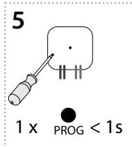
Press of programming button on receiver RFSA-62B shorter than 1 second will finish programming mode. The LED lights up according to the pre-set memory function.
