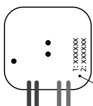
Addresses listed on the front side of the actuator are used for programming and controlling the actuator and individual RF channels by control units.
