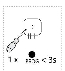
Channel selection is done by pressing the PROG buttons for 1-3s. After button release, LED is flashing indicating the output channel: red(1) or green (2). All other signals are indicated by corresponding color of LED for each channel.
