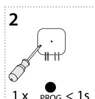
Pressing the programming button on the RFSA-62B receiver for less than 1 second will finish the programming mode, this will reverse the memory function. The LED lights up according to the current pre-set memory function. The set memory function is saved. Every other change is made in the same way.
