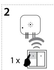
Select and press one button on wireless switch, to this button will be assigned function Button.
