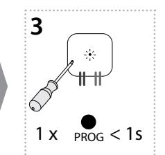
Press of programming button on receiver RFSA-62B shorter than 1 second will finish programming mode. The LED lights up according to the preset memory function.
