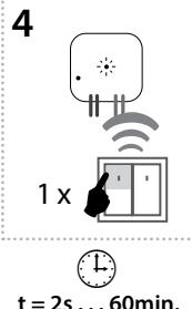
After the desired time has elapsed (range of 2s...60min), the timing mode ends by pressing the button on the RF transmitter, to which the delayed return function is assigned. This stores the set time interval into the actuator memory.
