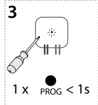
Press of programming button on receiver RFSA-62B shorter than 1 second will finish programming mode. The LED lights up according to the preset memory function.
