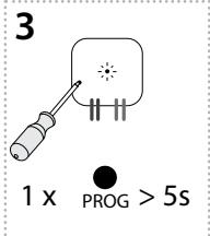
Press of programming button longer than 5 seconds, will activate actuator into timing mode. LED flashes 2x in each 1s interval.Uponreleasingthe button, the delayed return time starts counting.
