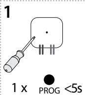
Press of programming button on receiver RFSA-62B for 3-5 second will activate receiver RFSA-62B into programming mode. LED is flashing in 1s interval.
