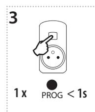
Press of programming button on receiver RFSC-61 shorter than 1 second will finish programming mode. The LED lights up according to the pre-set memory function.
