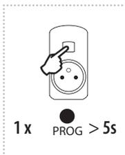
By pressing the programming button on the actuator for 5 seconds, deletion of one transmitter activates. LED flashes 4x in each 1s interval.
