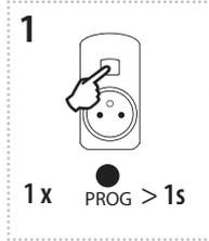
Press of programming button on receiver RFSC-61 for 1 second will activate receiver RFSC-61 into programming mode. Red LED is flashing in 1s interval.
