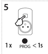
Press of programming button on receiver RFSC-61 shorter than 1 second will finish programming mode. The LED lights up according to the pre-set memory function.
