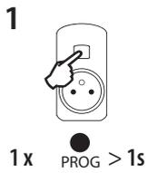
Press of programming button on receiver RFSC-61 for 1 second will activate receiver RFSC-61 into programming mode. LED is flashing in 1s interval.
