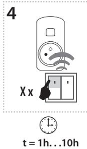
By the number of presses of the selected RF transmitter button, set the required delay (1 press - 1h, ... 10 presses - 10h). Each press on the RF transmitter is indicated by a flash of the LED on the socket RFSC-61.
