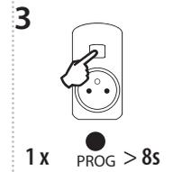
Pressing the PROG button for longer than 8 seconds brings the socket into the timing mode. The LED will give a single flash 3x and a double flash 3x, then goes out.
